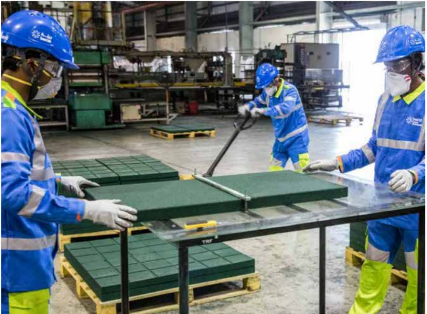
Figure 5: Rubber tiles produced from recycled tyres, at Bee'ah's Tyre Recycling Facility.
